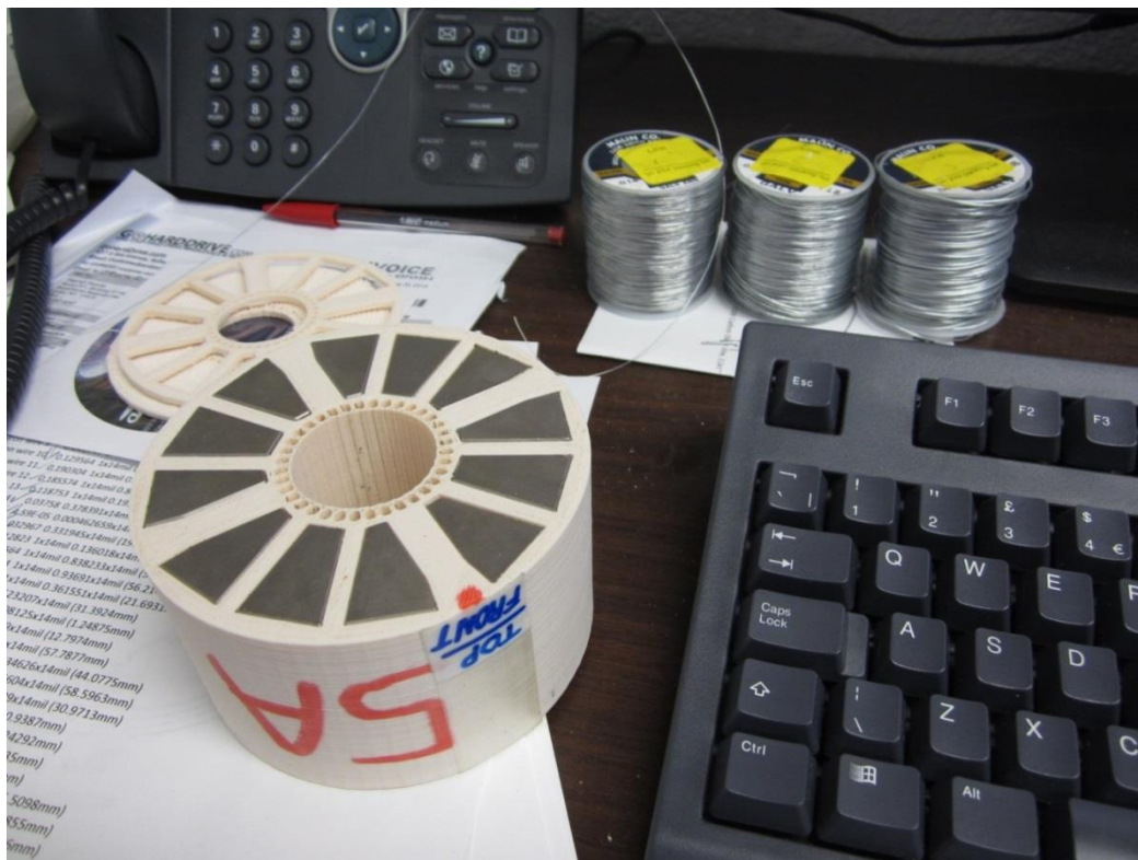
Figure. The pieces of the eRHIC LDRD Halbach magnet placed in a new 3D-printed holder to form magnet “5A”. This is a corrected Halbach quadrupole whose holder incorporates holes for iron shims to be placed around the inside of the bore (iron wire grades shown in background).
